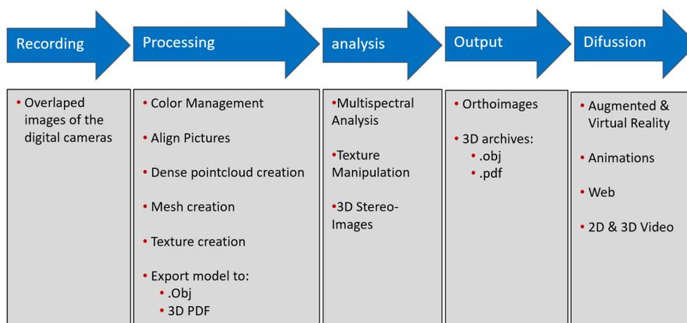
Fig. 5. Photogrammetric Processing Stages.
