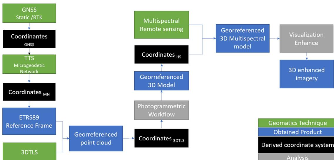
Fig. 1. Geomatics workflow diagram.
